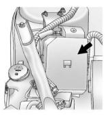
To uncover the remote positive (+) terminal, remove the fuse block cover. You should always use the remote positive (+) terminal instead of the positive (+) terminal on the battery.
